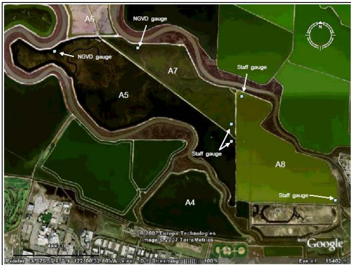
Figure 2: Water Level Gauge Locations
